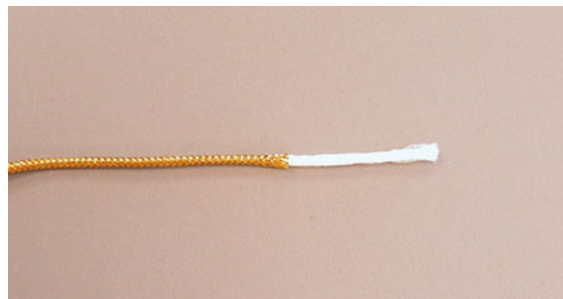
Figure 10.73 Exposing core of decorative piping.
