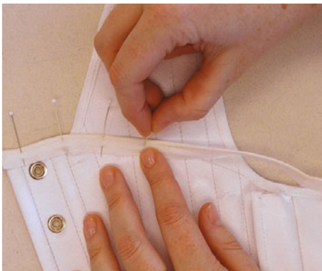
Figure 10.36 Pinning piping in place.
