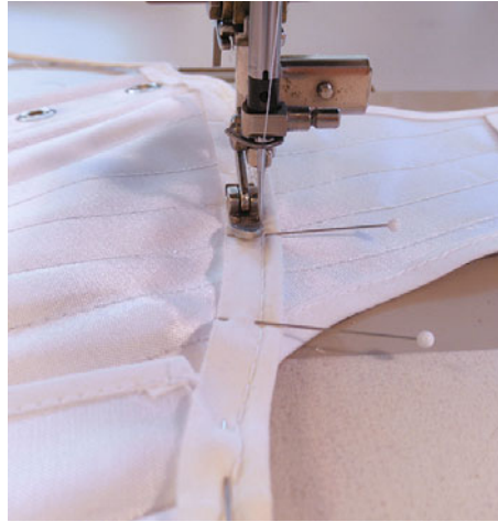
Figure 10.37 Stitching piping in place.
