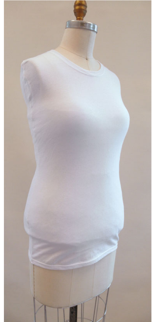
Figure 6.6 Covering the form.
