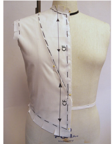
Figure 11.11 Completed doublet front with inset piece.
