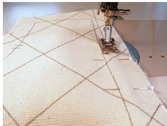
Figure 11.35 Flat lining layers together.
